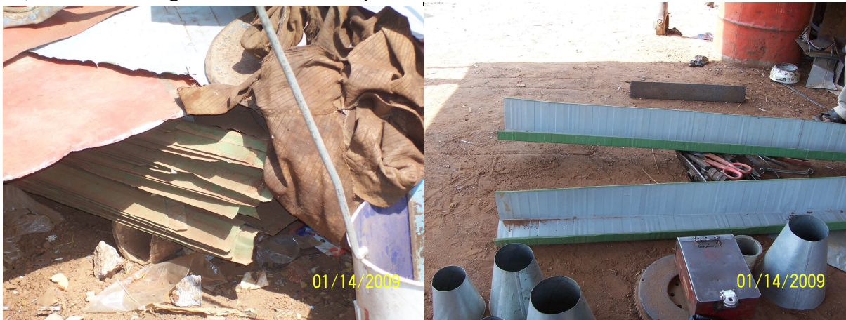
Figure 34: Fuseni Gutter Operation: steel sheeting from Accra (left), gutters and downpipe attachments (right)
