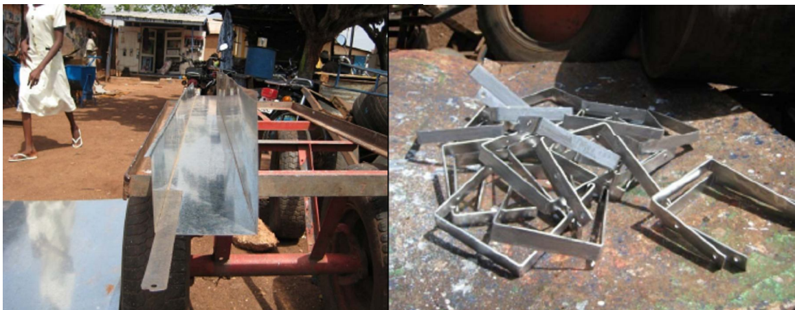
Figure 35: PHW Bent Steel Sheet Gutter Construction
